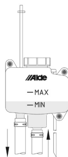
Fluid level in cold system
