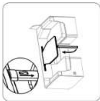
2 Locate the button to release the leg. fold the leg back 90 degrees until it locks below the table
