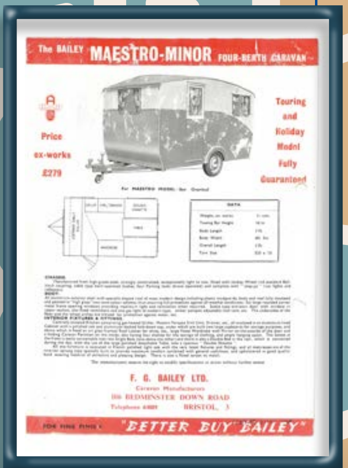
The four berth Bailey Minor only weighed 558kg, making caravan holidays accessible to a wider range of car owners.
