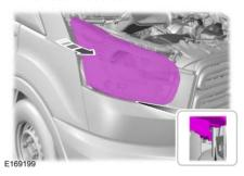
Pull the headlamp toward the front of your vehicle to disengage it from its locating points and then lift the headlamp up.
