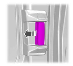
Pull and release the door handle to open the sliding door.
