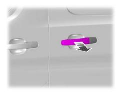
Pull and release the exterior door handle to open the sliding door.
