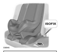
**WARNING:** Use an anti-rotation device when using the ISOFIX system. We recommend the use of a top tether or support leg.
