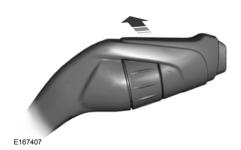
Push the lever away from you to operate the rear window washer. When you release the lever, the wiper operates for a short time.
