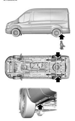
Position the vehicle jack under the rear leaf spring directly behind the rear wheel.
