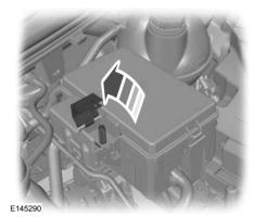
2. Lift up the battery positive connection point cover. For item location, refer to the appropriate under hood overview. See **Maintenance** (page 252).
