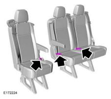
With the seat occupied, pull the lever or strap, or press the button to recline or raise the seatback.
