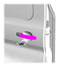
Pull and release the exterior door handle to close the sliding door.
