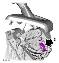
2. Locate the brake shift interlock lever.
