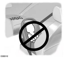
WARNING: Extreme Hazard! Never use a rearward facing child restraint on a seat protected by an active airbag in front of it. Death or serious injury to the child can occur.
