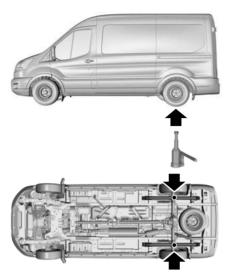
Position the vehicle jack under the rear axle.
