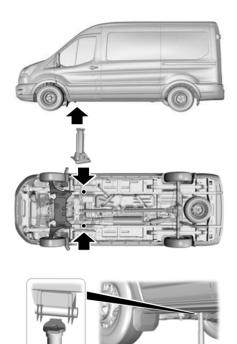
Position the head of the vehicle jack under the protrusions at the rear of front sub-frame.
