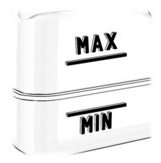
If the power steering fluid level is below the **MAX** mark, add power steering fluid that meets the correct specification.
