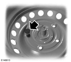
5. Remove the retaining nut to release the spare wheel bracket.
