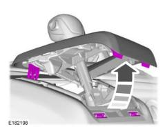
1. Using a flat-bladed screwdriver, remove the panel.
