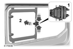
1. Press the unlock button to release the catch.
