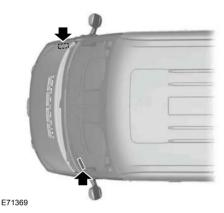
The vehicle identification number is located on the left-hand side of the instrument panel. You will also find it stamped into the right-hand front wheel arch.
