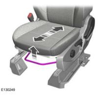
**Note:** The driver seat has removable stop bolts on the track to enable access to the vehicle battery. See **Changing the 12V Battery** (page 261).
