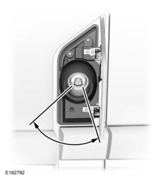
5. Operate the fuel pump nozzle within the area shown.
