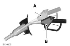
4. Hold the fuel pump nozzle in position B when refueling. Holding the fuel pump nozzle in position A could affect the flow of fuel and shut off the fuel pump nozzle before the fuel tank is full.
