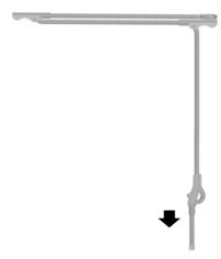
Insert the square end of the wheel brace or the short arm of the jack handle into the socket. Turn counterclockwise until the spare wheel rests on the ground and the cable is loose.
