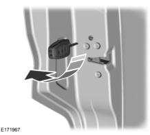
When there is no power to your vehicle, slam locking allows you to lock a door automatically when you close it. You can manually lock the front passenger door, sliding doors and rear cargo door using the key.
