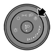
**Note:** When you switch the autolamps on, the headlamps turn on within 10 seconds of switching the wipers on.
