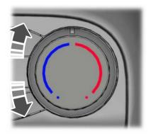
Turn the temperature control counterclockwise for cooler temperature settings.
