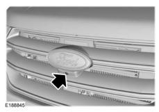
The front view camera is located in the grille. It provides a video image of the area in front of your vehicle. It adds assistance to the driver while driving forward at low speeds.
