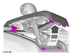
1. Using a flat-bladed screwdriver, remove the panel.
