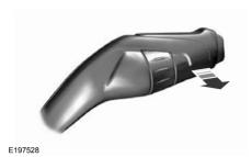
Pull the lever toward you to operate the windshield washers. When you release the lever, the wipers operate for a short time. A courtesy wipe occurs a short time after the wipers stop to clear any remaining washer fluid.
