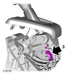
2. Locate the brake shift interlock lever.
