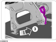
1. To remove the first seat, pull the strap located closest to the door.
