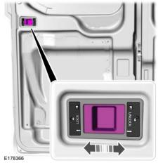
Slide the lever to release the catch and open the double rear doors fully.
