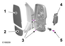
Remove the large mirror glass. Tilt the mirror glass fully up, pull the mirror glass toward you from the bottom.
