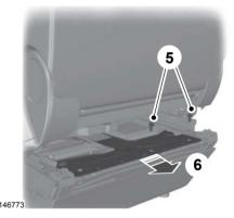
5. Remove the battery clamp and cover bolts.
