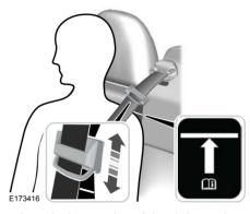
Adjust the lower edge of the slider so that it is above the white line.
