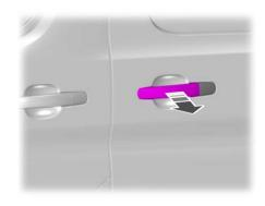
Pull the exterior door handle to open the sliding door.
