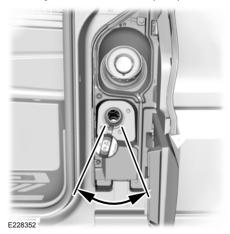
4. Operate the AdBlue® pump nozzle within the area shown.
