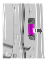
Pull and release the interior sliding door handle to close the sliding door.
