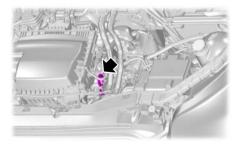
**WARNING:** Do not connect the negative jumper cable to any other part of your vehicle. Use the ground point.
