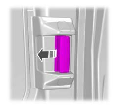
Pull the interior door handle to open the sliding door.
