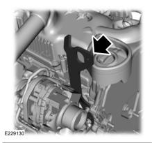
**WARNING:** Do not connect the negative jumper cable to any other part of your vehicle. Use the ground point.
