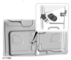
Pull the interior handle up to open the door in an emergency.
