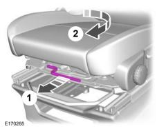
The seat can swivel through 180 degrees in an inboard direction. You may need to adjust the seat to allow sufficient clearance for it to swivel in a single motion.
