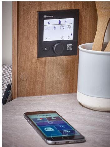
The Truma iNet System gives you remote access to your Truma or Alde boiler so you can control and monitor the heating and hot-water system wherever you are.
