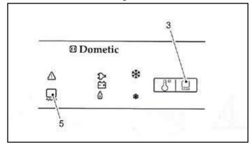
The frame heating is in operation with a presetting of 2 hours and switched off afterwards automatically. The frame heating can be deactivated every time by pressing the button (3).
