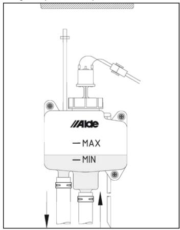
For manual filling, unfasten the expansion tank nut (R) and slowly pour the glycol mixture into the tank. Bleed the system and top up with more liquid if the level has fallen after bleeding. Bleed a newly- filled system regularly during the first days the heating system is in operation.
