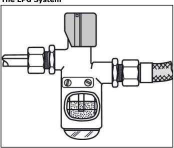
The LPG system should be checked regularly by a professional, who will ensure that there are no leaks from connections or hoses. LPG hoses should be changed according to national regulations, maximum of five years. Check the date stamp on the hose. Hose has a propensity to dry out and crack. To increase safety, we recommend fitting an Alde leak gauge, type 4071, as close as possible to the pressure reduction valve.
