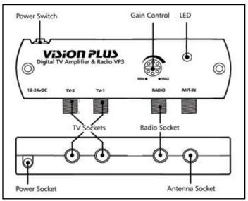
UHF 470-860 MHz Frequency Range: FM 88-108 MHz DAB 175-230 MHz Antenna Forward Gain 7db Amplifier Gain 16db Gain Adjustment 15db Noise Figure 2.8 db Output Impedence 75 ohms Output 95 dbuv Power Supply 12-24 vDC Power Consumption 55ma
