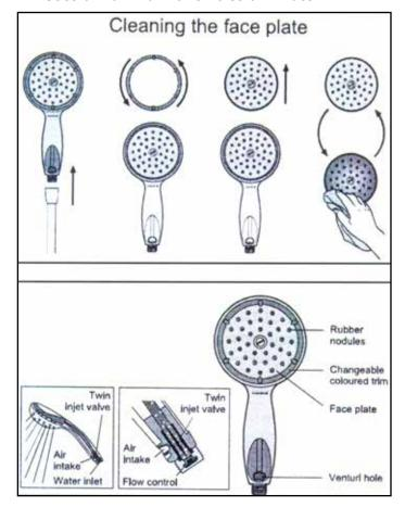
After showering when the shower is turned off, your ecocamel shower head simply drains off any excess water through the air intake
