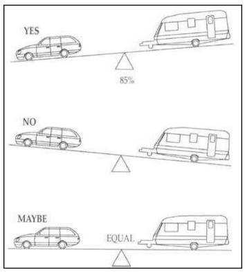
It should be noted that with certain layouts or models it may be necessary to load heavy items, such as awnings in the middle of the floor to achieve an acceptable and safe nose weight. It may not be possible to achieve the desired nose weight with all items stored 'out of sight' in lockers and bed boxes (bunks.)
