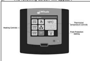
Fig 3: Space Heater Screen display.
