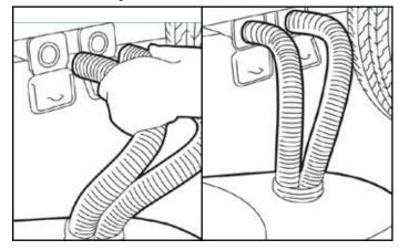
When setting up your caravan short pieces of waste pipe hose should be fitted to the wastewater outlets to direct the water into a suitable container. These are both available from your caravan retailer.
