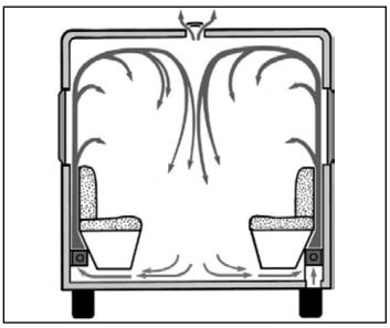
While camping during the winter, ensure that the flue is kept clear of snow and ice, since the inlet air to the LPG boiler enters through the flue. Do not start the LPG boiler until the flue is completely free of snow.
