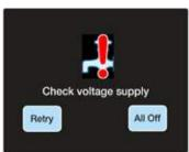
Ensure voltage is above 10V and below 15V at the heater.
