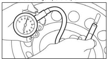
Consult your tow vehicle manufacture for the correct tow vehicle tyre pressures for towing.
