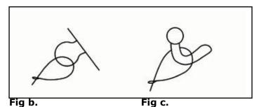
Fixed ball- Loop the cable around the neck of the tow ball. If you fit the cable like this, use a single loop only. See Figs. b and c.
