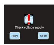
Ensure voltage is above 10V and below 15V at the heater. This can be done by recharging the battery. "Check outside flues for blockages"
