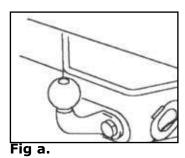
Pass the cable through the attachment point and clip it back on itself. (fig a)
