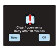
The heater has overheated due to the vents being either closed or blocked – for example with a cushion or bag. Remove the blockage and open any closed vents. Leave the heater for 10 minutes to cool down, then try again.
