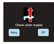
The heater isn't completely full of water. Run the pump with one hot tap open until water flows smoothly out of the tap. Wait at least 5 to 10 minutes to allow the heater to cool before pressing "Retry".
