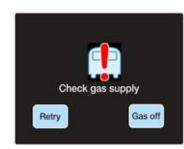
Make sure there is gas in the bottle and no blockage in the gas line. At temperatures below 5°C use Propane rather Butane. **Press** than "Retry" once the checks are complete. If there is a problem with the gas supply which can't be dealt with immediately, select an electric-only heating option instead.
