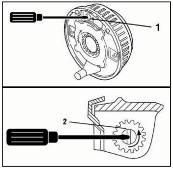
vi. Slacken off the starwheel adjuster until the road wheel turns freely in the forward direction (fig. 9). vii. Check the adjustment at the end of the brake cable where it is secured to the abutment (bracket) welded to the centre of the axle. When the inner cable is pulled out it should extend between 5 and 8 mm (fig. 8). (On tandem axles a double abutment
