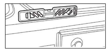
The positioning of the jockey wheel can be used to help level the caravan.
