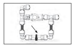
4. Turn the 2-way valve to the open position shown below.
