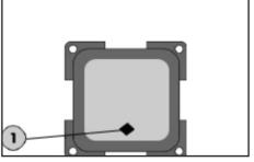
1. Button to check the voltage (in volts) of the connected 12v battery.
