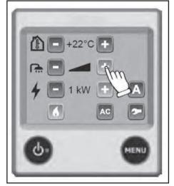
Volume bar full. Central heating circulation is disabled for 30 mins. Hot water is heated to greater than 65°C. After 30 mins the system reverts to Hot Water Normal. Adjust by pressing plus or minus button.
