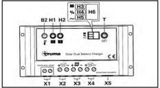
H1 LED: Function display battery 1 H2 LED: Function display battery 2 H3 LED: Battery type- AGM, gel, liquid H4 LED: Charging current distribution H5 LED: PWM charging frequency H6- shows the values of H3, H4, H5 as numbers T Query/change operating mode B2 Internal Temperature sensor X1 Connection for temperature sensor B1 X2 Connection for battery 1 X3 Connection solar module X4 Connection for battery 2 X5 Connection (RJ-45) for remote display (optional)
