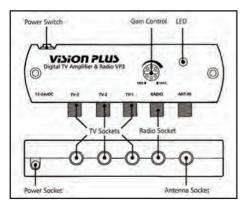
Frequency Range UHF 470-860 Mhz Frequency Range VHF 40-230 Mhz Frequency Range FM 88-108 Mhz Amplifier Gain Max 18db Gain Adjustment 15db Flatness +1.5db Noise Figure 2db Output Impedance 75ohms Signal Handling 80dbuv Power Supply 10.8-28v DC
