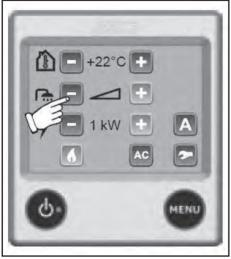
Volume bar empty. No attempt is made to heat hot water specifically. This saves energy when the freshwater is drained down.
