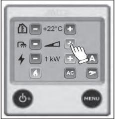
Volume bar half full. Hot water is heated to greater than 50°C. NB: If circulation pump is set to Continuous, this option will not be available.
