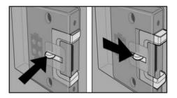
Release the locking mechanism of the door lock by pushing it in and moving to the front. If the door is shut in this position, a small gap is nevertheless kept open to prevent formation of mildew (Fig. 38-39).
