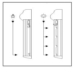
Retensioning. If this is required on either blind the screw head located on the side of the roller should be turned once and the blind tested. If the tension is still not correct further turns may be required.
