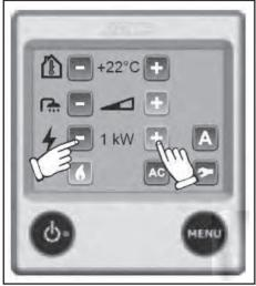
Check that 230v supply is displayed on the Standby Screen. The Alde boiler is programmed to use power economically and there are times when it may use no power at all, even if set to 3kW.
