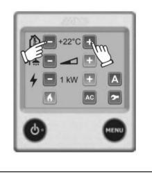
The desired room temperature can be set from 5°C to 30°C, in 0.5°C increments.
