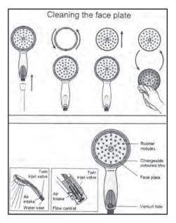
After showering (when the shower is turned off) your Ecocamel shower head simply drains off any excess water through the air intake. Clean your Ecocamel shower head with a damp cloth. Do not use any abrasive or chemical cleaners. Should any scale build up on your shower head's spray plate you can de-scale it by rubbing the nozzles with your thumb.
