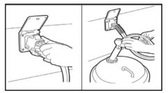
Open the kitchen hot tap and allow the system to purge itself of air and is a steady flow of water is present. This will also fill the water heater ready for heating.
