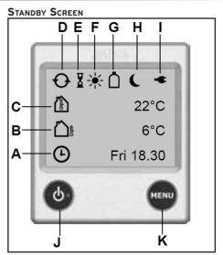
The Standby Screen is displayed after the Splash Screen. This screen contains useful information about the status of your heating system.
