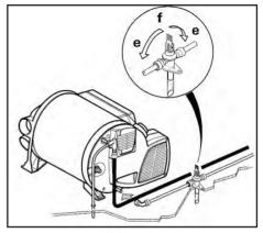
e. Lever position "closed" f. Lever position "drain"
