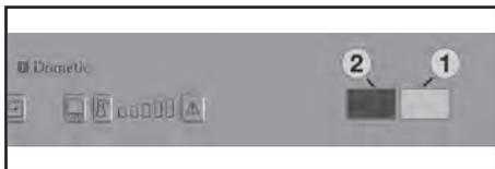
Depending on the door opening direction, there are two LEDs on the left or right edge of the control panel. The outer LED 1 indicates that the refrigerator is operational (blue). The other LED 2 lights red in the event of a fault.
