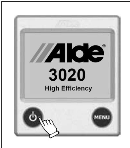
To start the system, press the Power button on the control panel.
