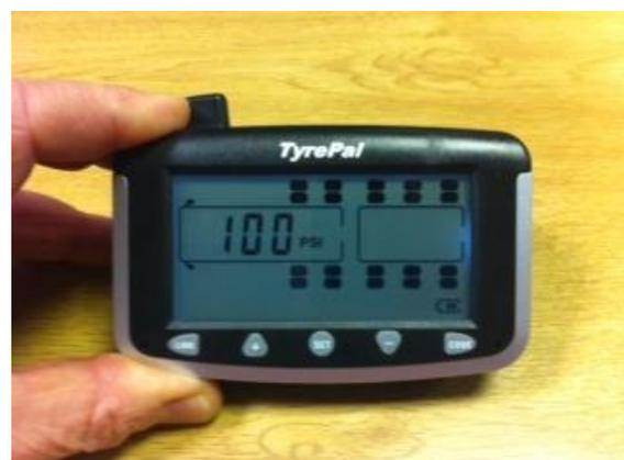
To adjust the low pressure alert level, press the + or – button to adjust the monitor to the required alert level for that axle.
