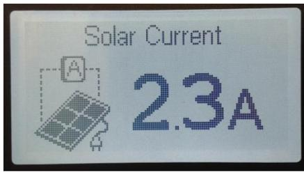
This page displays the amount of current that is being generated by the solar panel. A solar regulator is required to drop down the solar panel voltage to battery safe levels.
