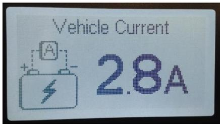
This page displays the amount of current being drawn from the Vehicle Battery, when the Vehicle Battery is being charged a lightning icon is displayed inside the battery. A higher current will draw will drain your battery faster.
