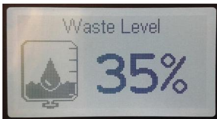
This page displays the current waste water level inside the waste tank as a percentage. If the “High Waste” notification is enabled the user will receive a notification when their waste tank fills up over 90% by default.
