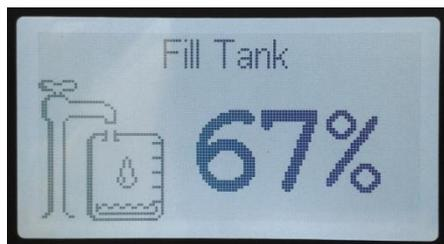
This page is the fill tank screen. When the external pump is connected to the inlet and to an external water source pressing the
