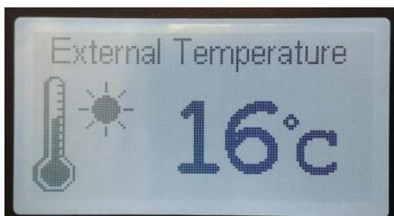
This page displays the external temperature, it is measured by a sensor placed on the outside of the van (usually on the underside).
