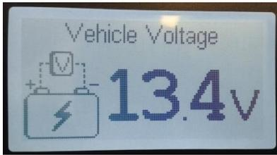
This page displays the vehicle battery voltage. If a 230V mains supply is connected then the charging voltage of the vehicle battery will be displayed. If the vehicle battery is being charged then a lightning icon will appear in the battery.
