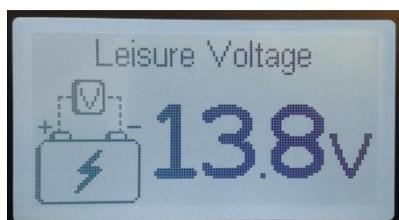
This page displays the leisure battery voltage. If a 230V mains supply is connected then the charging voltage of the leisure battery will be displayed. If the leisure battery is being charged then a lightning icon will appear in the battery.
