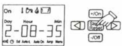
If the power to the panel is broken and the battery backup is not connected, the clock must be set again.
