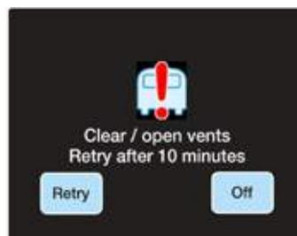
The heater has overheated due to the vents being either closed or blocked - for example with a cushion or bag. Remove the blockage and open any closed vents. Leave the heater for 10 minutes to cool down, then try again.
