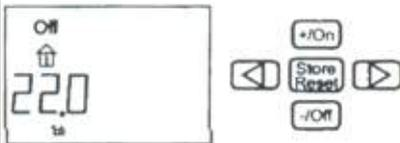
When external start is activated the heater will start with the latest settings and "ON" (main breaker) comes on. If 12V is not connected to the heater, the display will not light up until 12V is connected. The external start function is still activated.
