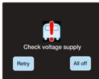
Ensure voltage is above 10V and below 15V at the heater. This can be done by recharging the battery. "Check outside flues for blockages"
