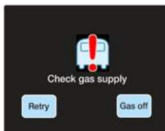
Make sure there is gas in the bottle and no blockage in the gas line. At temperatures below 5°C use Propane rather than Butane. Press "Retry" once the checks are complete. If there is a problem with the gas supply which can't be dealt with immediately, select an electric-only heating option instead.
