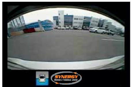
Full-screen ultra wide-angle front/rear views (selectable with command switch)
