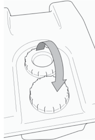
Fig. 4 Swap caps to prevent water spillage in transit.
